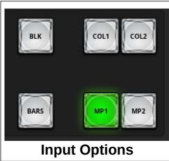
In addition to the 8 video inputs, the ATEM has 6 other options; **BLK** (black), **BARS** (color bars), **COL1** and **COL2** (solid colors), and **MP1** and **MP2** (frame stores). These are available in both the Preview and Program sections of the ATEM Control Panel.
